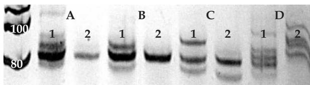
**Figure 6.** Optimized TCR $\gamma$  protocol tested in T-cell lymphoma cases. A, B, C: monoclonal pattern; D: polyclonal pattern. (1) template dilution 1:10; (2) template dilution 1:100. Dominant reproducible band within the expected size range is indicative for monoclonal rearrangement in lanes A, B, and C. Polyclonal pattern is seen in lane D with multiple inconsistent sized bands.
